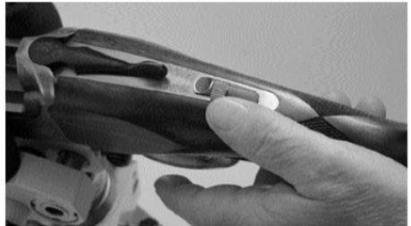
1. The safety mechanism on your shotgun is located on the action tang immediately behind of the top lever
